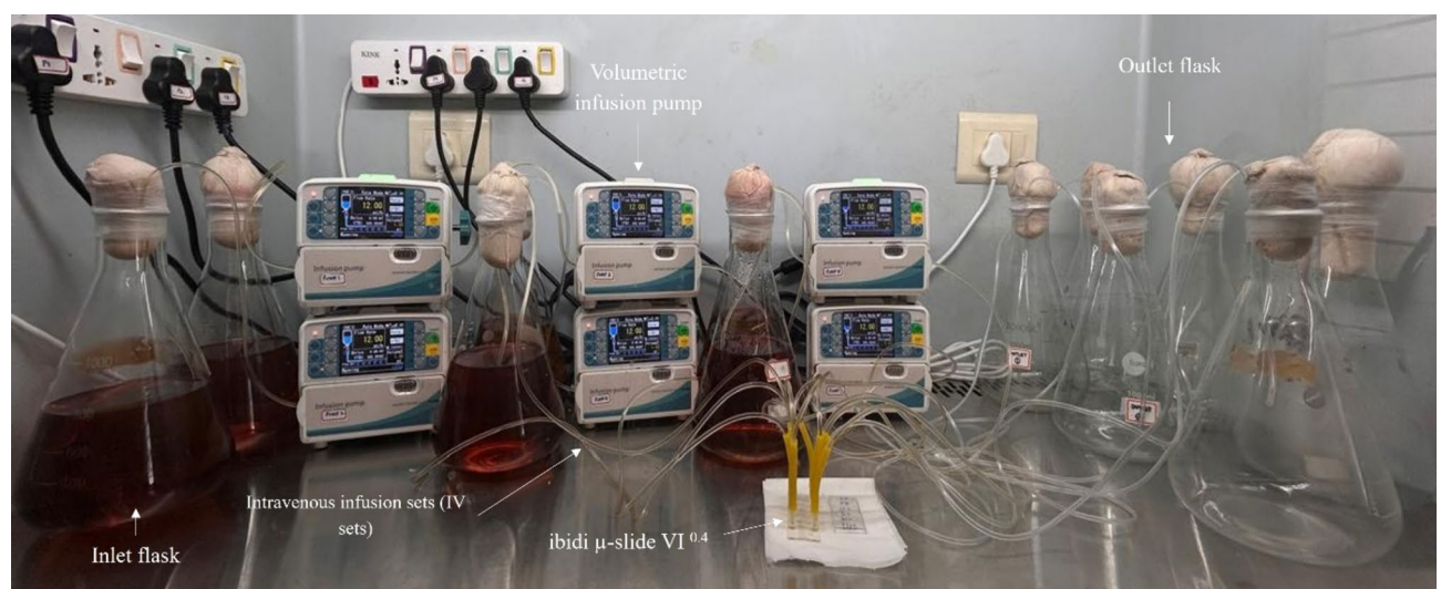
Fig. 2. Flow system: The flow system was set up in a biosafety cabinet to maintain sterility of the experiment. The actual experimental system containing the inlet flasks containing sterile BHI media, the IV sets used for flowing media to the channel of the ibidi \mu -slide VI 0.4 , and the outlet flasks to collect the out flown media.
